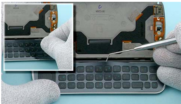
39) Start releasing the QWERTY KEYMAT with the dental tool. Remove the keymat by peeling it as shown.
