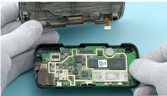
15) Separate the upper part and the B-cover with the engine board.
