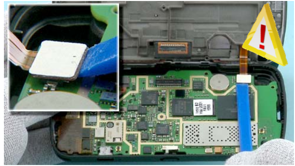
14) Then open carefully the Q-ROCKER FPC ASSEMBLY CONNECTOR with the SS-93.
