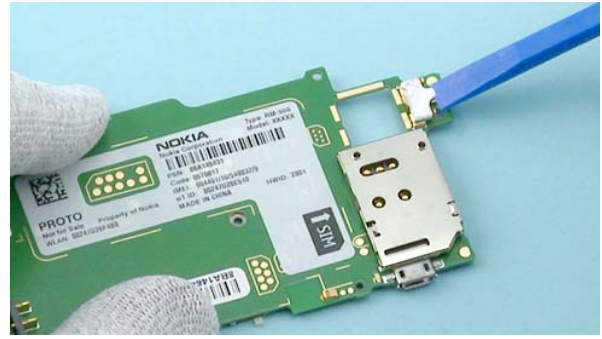
26) Release the HEAT SINK ASSEMBLY with the SS-93 and then remove the assembly.
