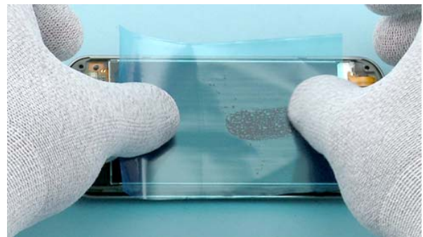
34) Remember to protect the LCD with protective film.
