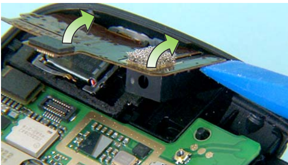
17) Next, lift up the AUDIO ASSEMBLY with the SS-93.
