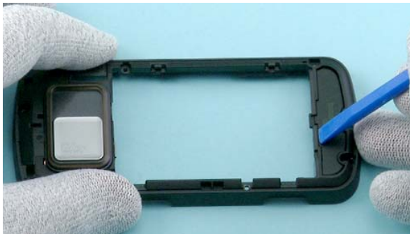
27) Use the SS-93 to detach the antenna assembly and then remove it.
