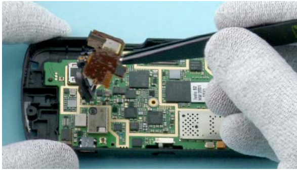
19) Remove the AUDIO ASSEMBLY and the IHF HOLDER ASSEMBLY with the tweezers.
