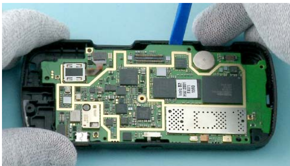
21) Release the engine board with the SS-93.
